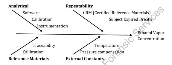
2.6.8 **Figure 1** is a cause-and-effect diagram showing the uncertainty sources incorporated into the budget for the breath alcohol reference materials. It applies to both the external standards and the instrument calibration and measurement process. There are four major components that contribute to the overall uncertainty, and they are broadly categorized as: analytical (Type B), repeatability (Type A), reference materials (Type B) and external constants (Type B).
