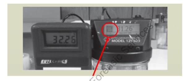
5.13 **STEP #10:** Insert the small, slotted screwdriver into the mode switch and press to advance to the VR2 *c*ircuit for the display/thermometer display (thermometer symbol to the left of the temperature reading).
